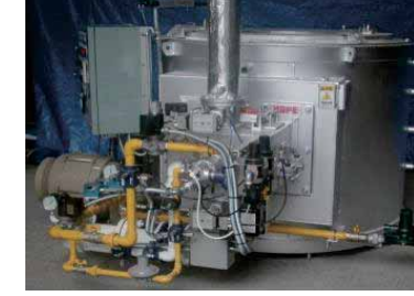
Regenerative Burners in industries, Toyotsu Machinery, Indonesia
